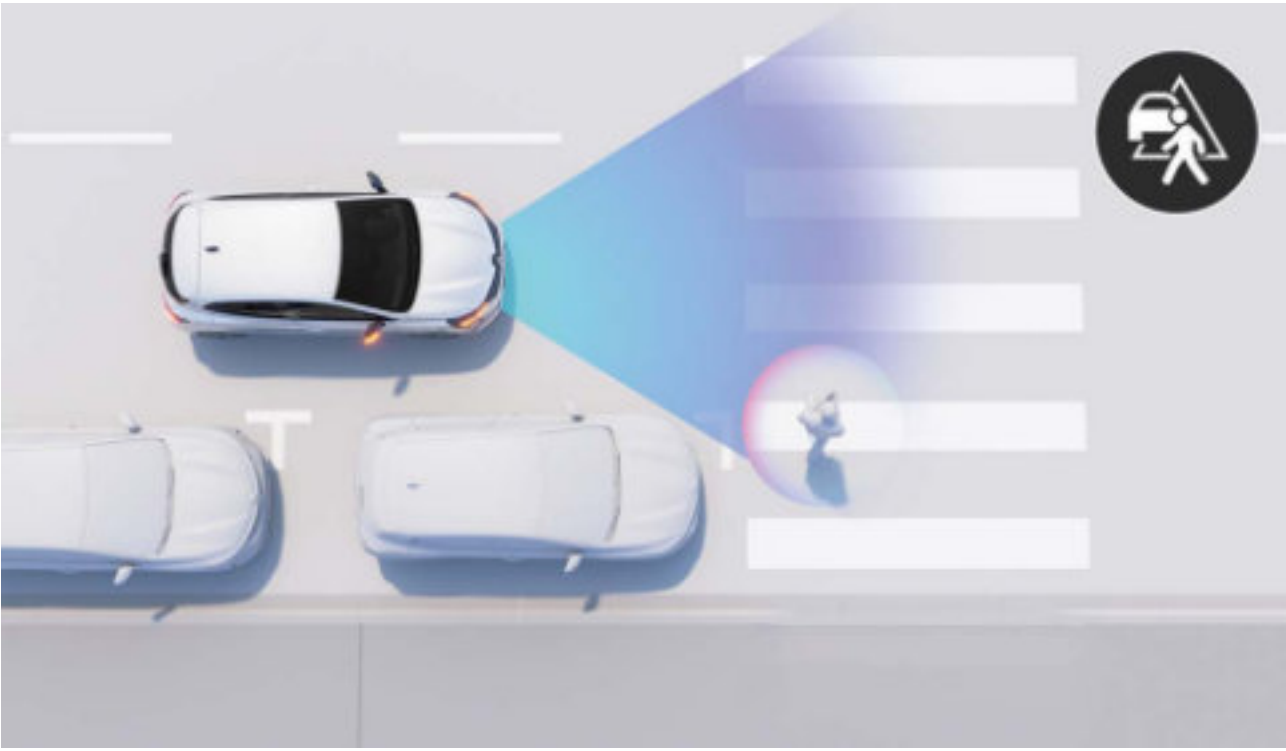
automatic emergency braking Warns the driver of an imminent risk of frontal collision with a stationary vehicle, at low speeds. Triggers automatic emergency braking to avoid or mitigate a collision.
