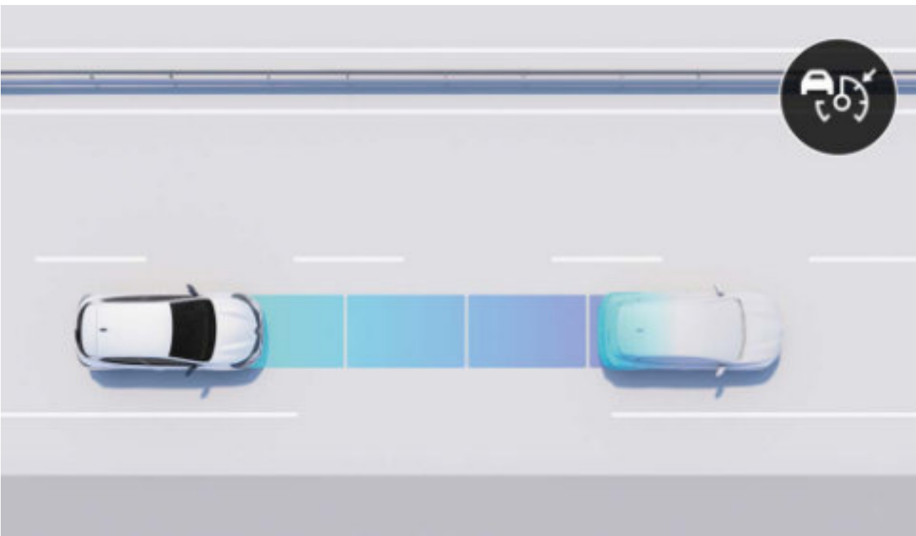
adaptive cruise control The system keeps a safe following distance from the vehicle in front of you. It activates the brakes if you get too close and accelerates when the road is clear again.
